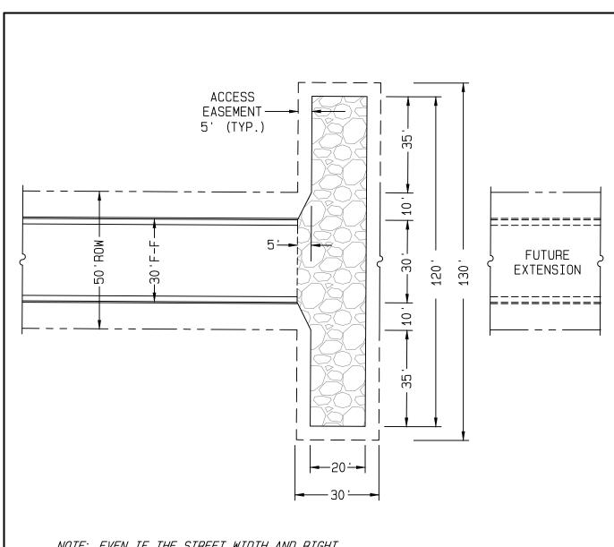
NOTE: EVEN IF THE STREET WIDTH AND RIGHT OF WAY ARE LESS THAN 30' AND 50' RESPECTIVELY, THE DIMENSIONS OF TEMPORARY TURN AROUND MUST STILL MEET THE OVERALL LENGTH AND WIDTH DIMENSIONS SHOWN.
