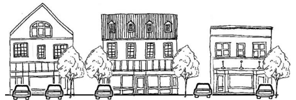
A consistent pattern of windows, floor heights, and building details should be maintained with new construction.
