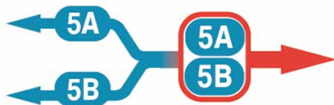
Figure 47: In the Concepts, "branch" routes combine to provide a higher frequency on their shared "trunk" segment. Such routes have the suffixes "A" and "B".
