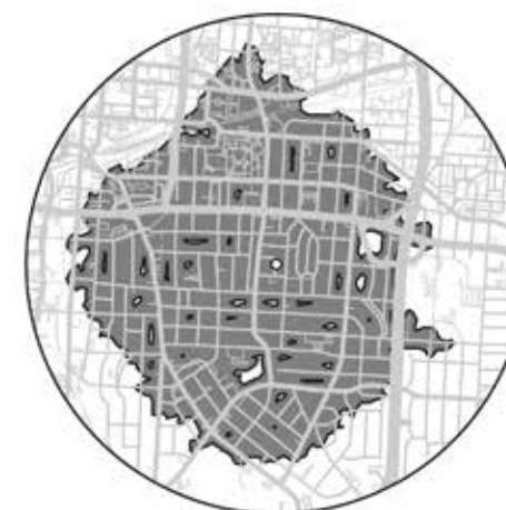
Continuous grids with many intersections and few barriers lead to high connectivity
