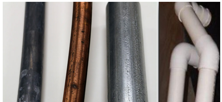
Sample Service Line Materials: lead, copper, galvanized steel, PVC/plastic
