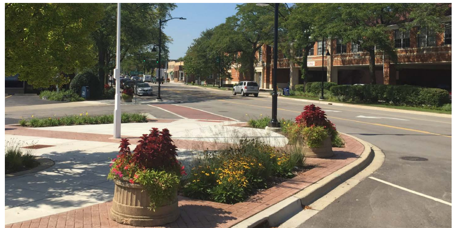
The above image depicts a traffic calming treatment at an intersection. This corner extension, also known as a pedestrian bump-out, forces drivers to slow as the road narrows and also reduces the distance for pedestrians to cross the street.
