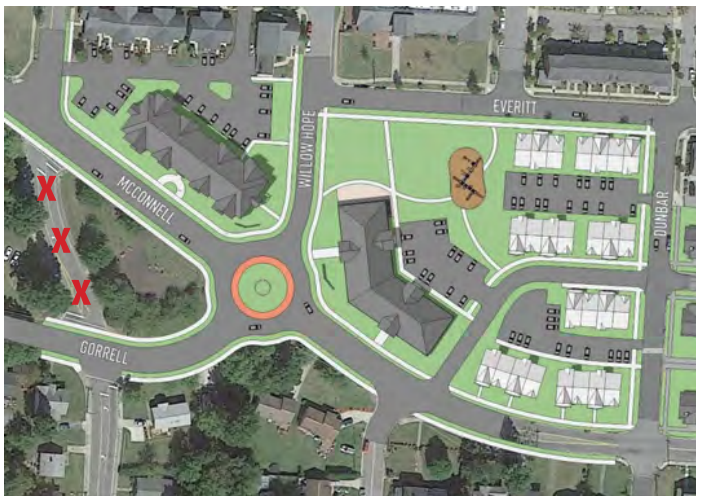
Figures 61 and 62: Gateway entry roundabout and red X's displaying partial elimination of Lincoln Street.
