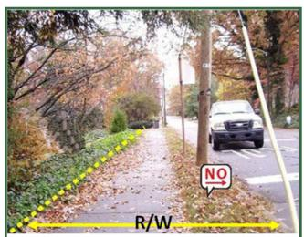
The sidewalk is behind the utility poles, therefore the backside of the sidewalk approximates the right-of-way line for purposes of enforcement. This is typical in many older neighborhoods. Signs must be behind the sidewalk in this example.
